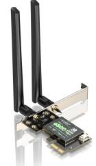
When used with a Wi-Fi 7 router, EP-BE9726 supports Multi-Link Operation (MLO)\* and up to ~6.5 Gbps theoretical throughput across 2.4 GHz, 5 GHz and 6 GHz bands.
