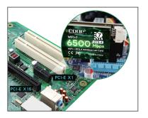
③. Find the 9-pin USB interface on the motherboard, insert the external wiring of the PCI-E card into the USB interface of the motherboard, and install the screws to secure the bracket
