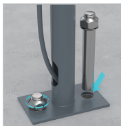
5. Installation to the pre-drilled holes on the floor
