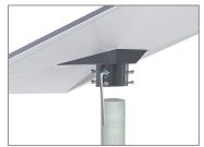
Adjust the screws to the size of the mounting bar
