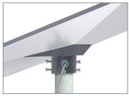
Attach to the uprights and tighten the screws.
