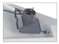
Pass the cable through the bracket and connect it to the machine.
